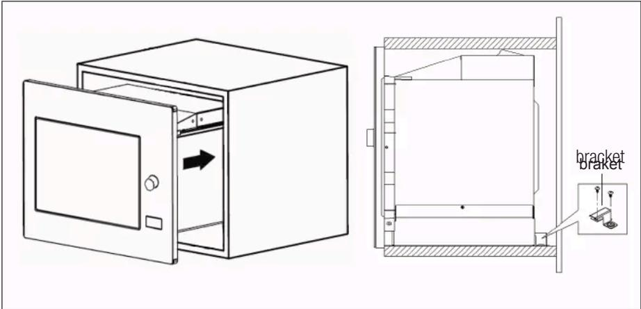
2. Open the door, fix the oven to the cabinet with Screw B through the installation hole. Then fix the trim-kit plastic cover to the installation hole.
